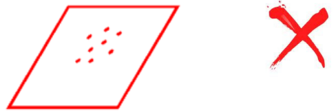
Probing points distributed non-uniformly measure the real shape incorrectly
