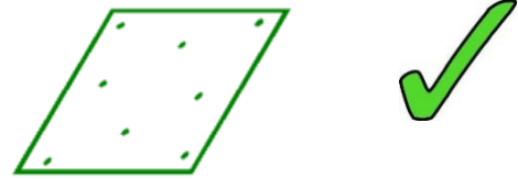
Probing points distributed uniformly measure the real shape correctly
