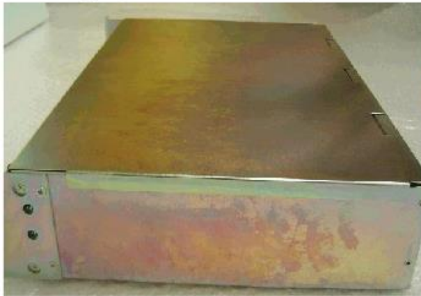
Fig. 1; This Finish Is Unacceptable
