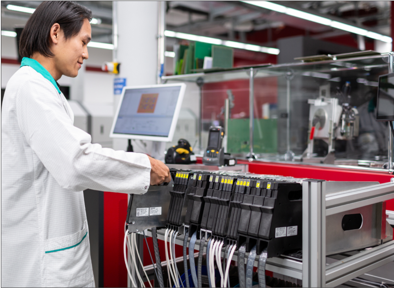
Active Feeder Rack: Kitted feeders that will soon be needed again are temporarily stored here. The LED signals immediately show employees which feeders are needed for the next setup. The target track of the new setup is also displayed.
