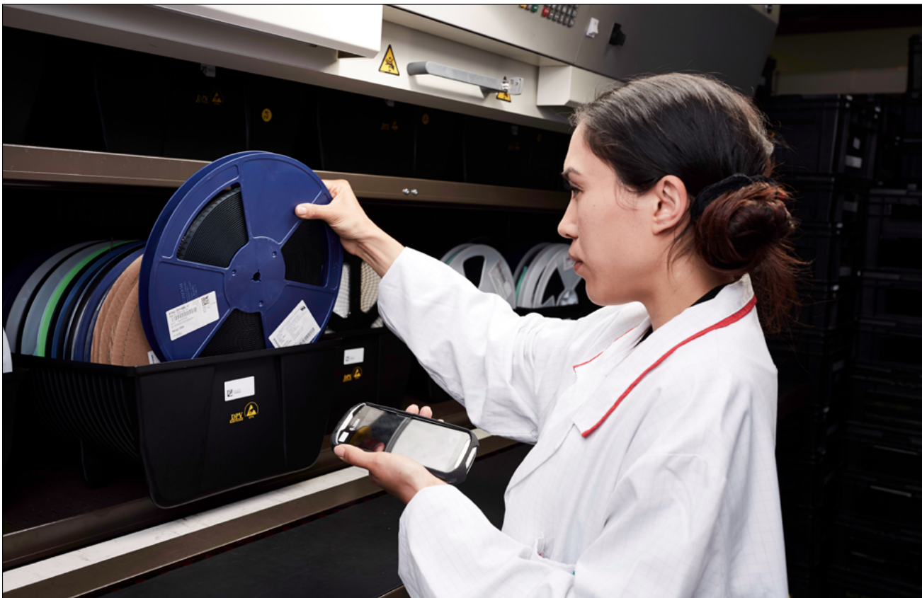
Software-supported material stock extraction: employees receive pick lists optimized by Factory Material Manager to their handheld devices and confirm the removal by scanning the UID.
