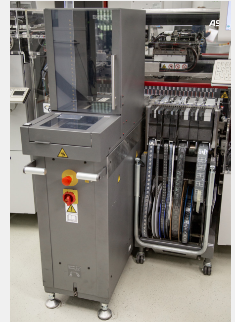
SIPLACE Waffle Pack Changer enables non-stop feeding of tray-based components in a compact, space-saving design.
