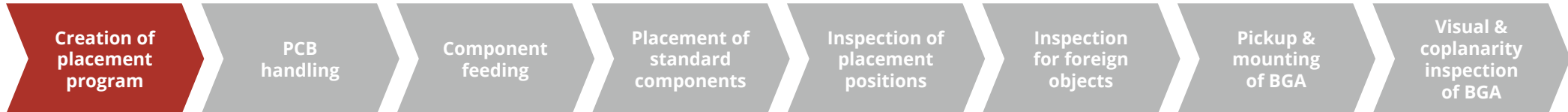
Import of ball position data at the station or offline station
