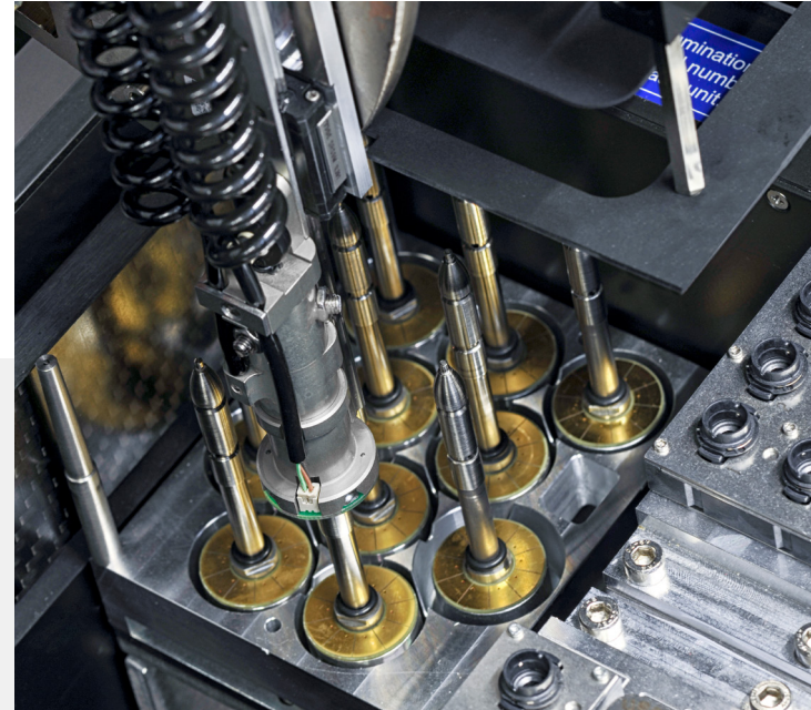
Automatic placement of support pins with continuous position monitoring
