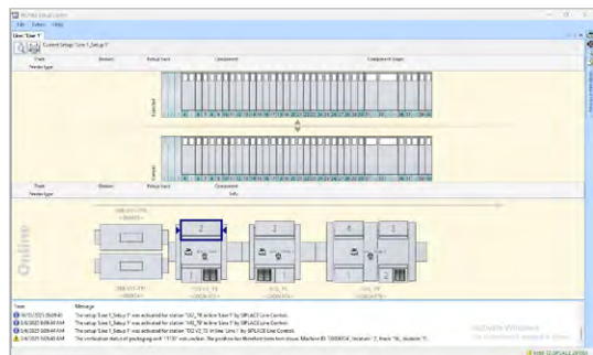
Detailed status view of tape feeders on SIPLACE placement machines
