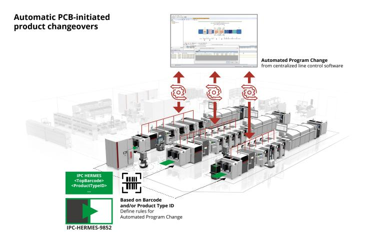
Automatic Program Change: Product information is forwarded from machine to machine via the standardized IPC-HERMES-9852 interface. Each station checks whether a program change is needed and automatically downloads the new program if necessary.
