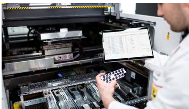
Operators can see at all times where individual nozzles are located, how many placement processes they have executed, their maintenance status, their faults and fault rates, when their last check was performed, and whether they are currently being blocked.
