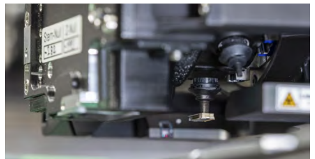
As the only direct physical interface with the component, the nozzle plays a critical role for the quality of the pickup and placement process.
