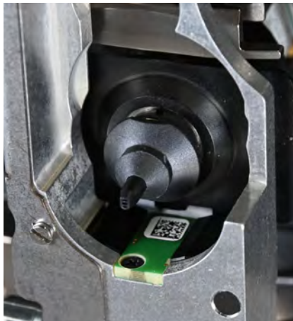
Nozzles are identified via RFID chips in the nozzles and RFID readers in the SIPLACE placement machines.
