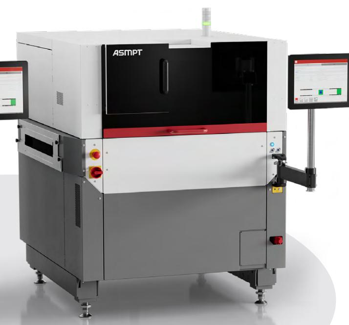
With its many interface standards, the DEK TQ printer platform fits seamlessly into the intelligent factory while its growing number of options automates setup changeovers and minimizes operator assists.
