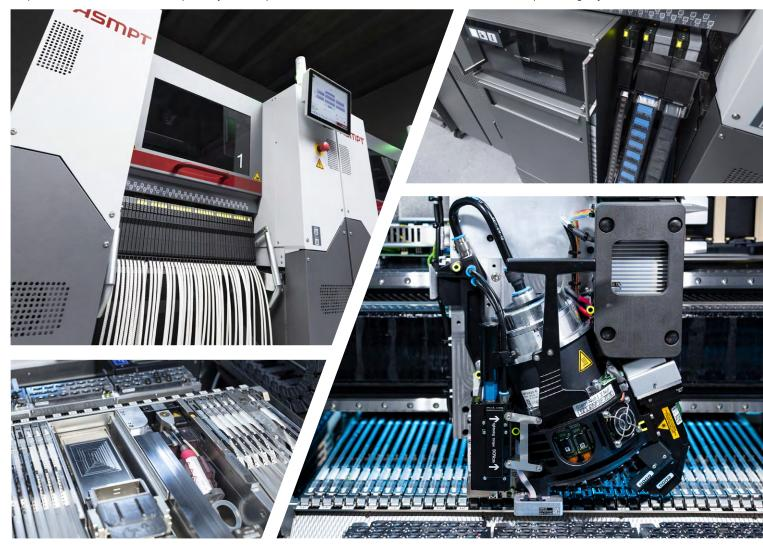
Fully compatible with all SIPLACE X feeders, Linear Dipping Unit, Power Connector, Glue Feeder, and Measuring Feeder.
