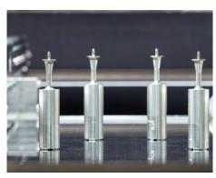
Smart Pin Support prevents PCB bending at critical points.
