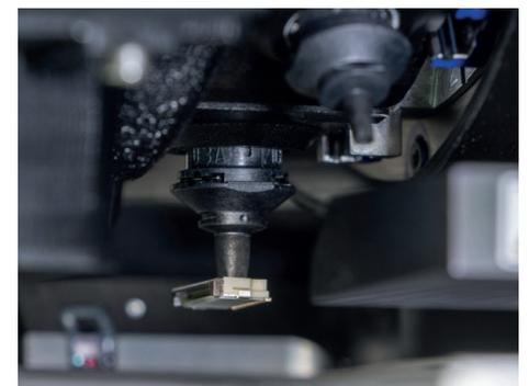
Rotatable nozzle segment precisely align with the components already during the pickup process.
