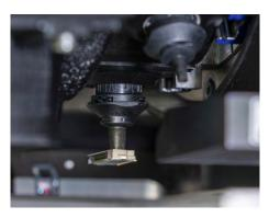
Rotatable nozzle segment precisely align with the components already during the pickup process.
