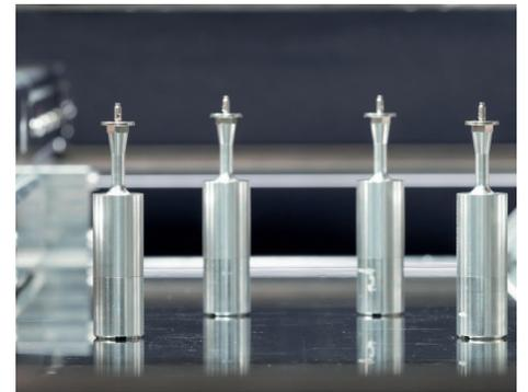
Smart Pin Support prevents PCB bending at critical points.
