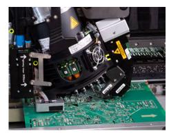
Peak performance of up to 52,500 cph in a compact footprint of only  $1.1 \times 2.4$  meters.
