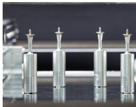
Smart Pin Support prevents PCB bending at critical points.
