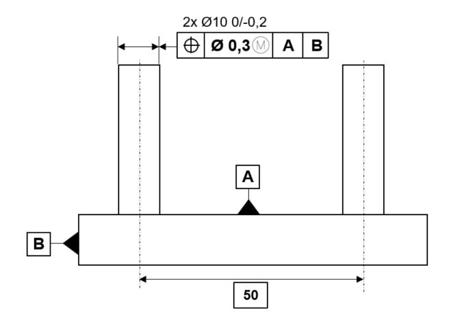
We consider the positional requirement for the pin in the above example. Initially, a positional tolerance of  $\emptyset$ 0.3 applies. Due to the operator of the maximum material condition, this tolerance increases depending on the actual value of the pin diameter  $\emptyset$ 10. The resulting positional tolerance is listed in the table below, depending on the actual pin diameter:
