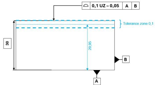
or clarification, the same part is shown below with a profile tolerance without the UZ modifier. Here, the resulting dimension is 30 +/- 0.05:
