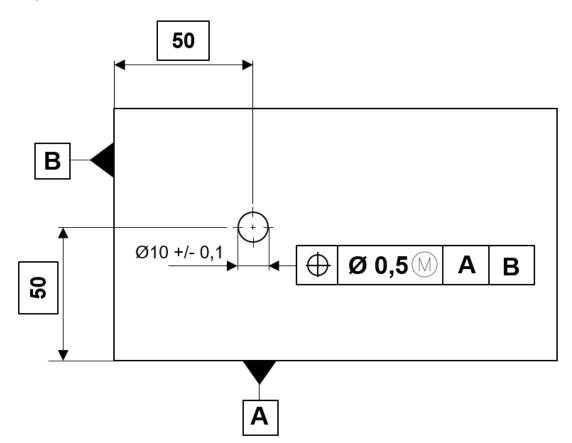
We consider the positional requirement for the bore in the above example. Initially, a positional tolerance of  $\emptyset$ 0.5 applies. Due to the operator of the maximum material condition, this tolerance increases depending on the actual value of the hole of diameter  $\emptyset$ 10. The resulting positional tolerance is listed in the table below, depending on the actual diameter:
