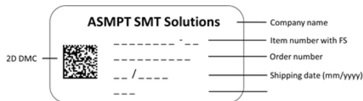
The 2D coding must be implemented as DataMatrix ECC 200 according to ISO/EN 16022.
