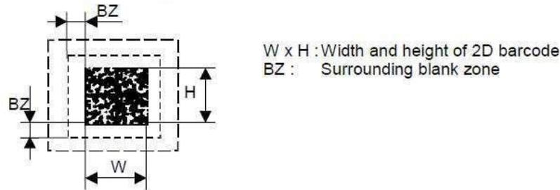
The blank zone (BZ) must be implemented as a function of the barcode resolution (X) as  $\geq 2X$ .
