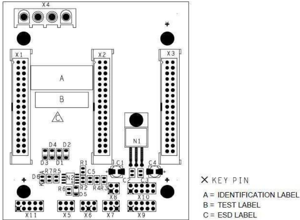
The locations of the labeling are defined in the board's component mounting diagram. Each location is identified with a letter code (A, B, C) and an outline.
