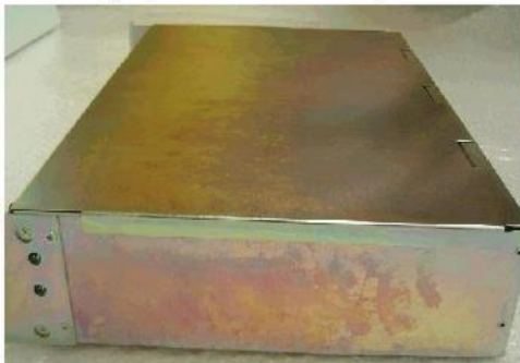
Fig. 1; This Finish Is Unacceptable
